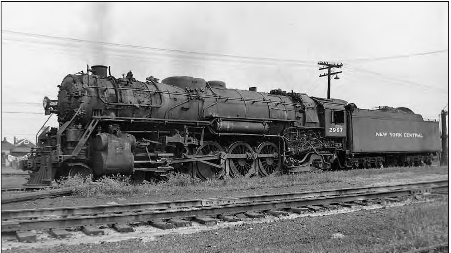
L-2d 2967 was less than two years away from retirement when photographed by the author at the Lansing, Michigan roundhouse in August of 1953. Built by Alco-Schenectady in November 1929, the beefy 4-8-2 will be retired in March 1955.
