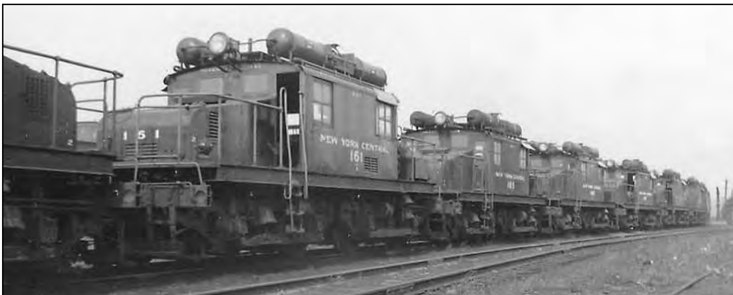
Also in March of 1954 Richard photographed a string of R-1 B+B electric motors awaiting disposition after being withdrawn from tunnel service in Detroit.
