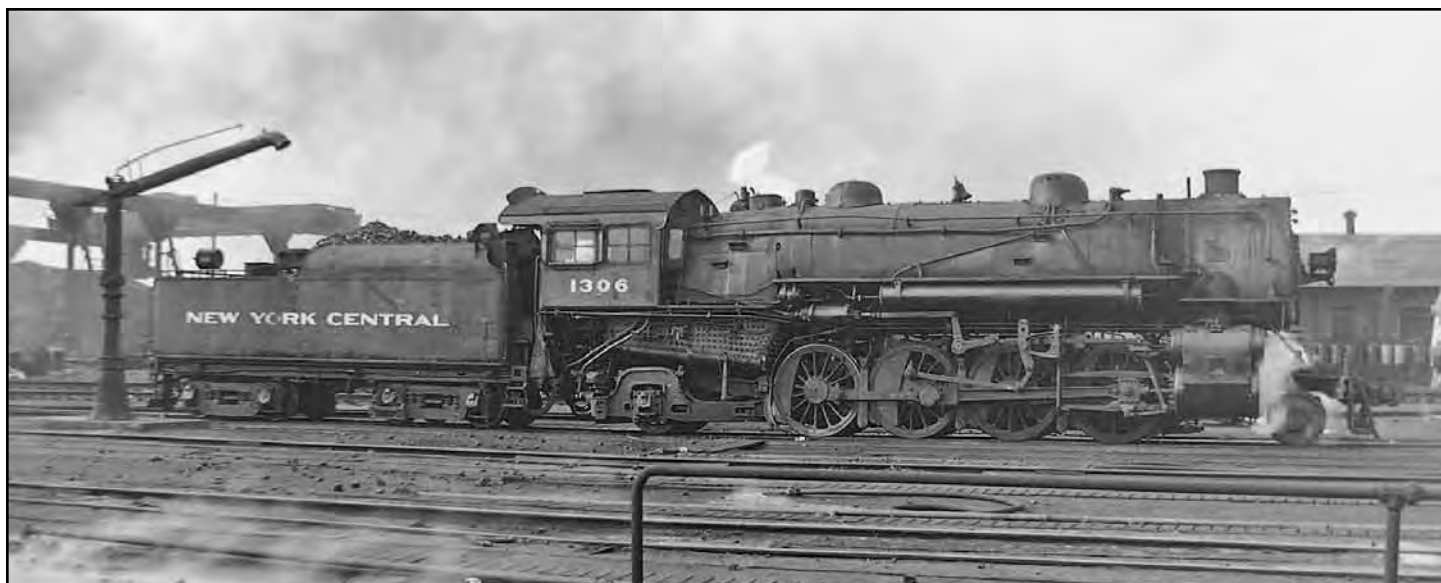
Visiting the engine terminal in Detroit in March of 1954, Richard photographed H-5j Mikado 1306 resting between transfer or local freight duties. This was one of twenty H-5's orphaned off the Boston & Albany following total dieselization of the New England carrier in 1948. She was built as B&A 1202 by Alco-Schenectady in December 1913, renumbered to NYC 1306 in April 1951, and will be retired in March 1955.
